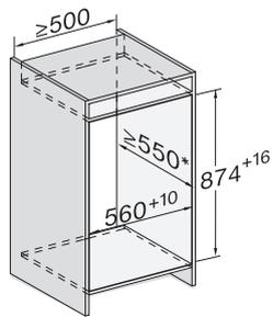
FNS7140B, FNS7140C, FNS7140D, FNS7140E, built-in (\*footnote) (installation drawings)
