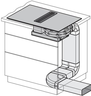
KMDA 7774, KMDA 7633 built-in version (Installation drawing)
