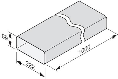
DFK-R1000, Flat-type ducting, 1000 mm, installation drawing
