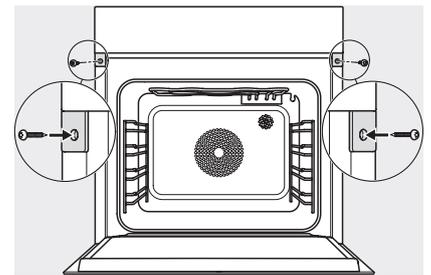
screw joint DGC XXL, installation drawing
