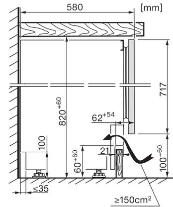
KWTUS7096E, Built-under, side view (installation drawings)
