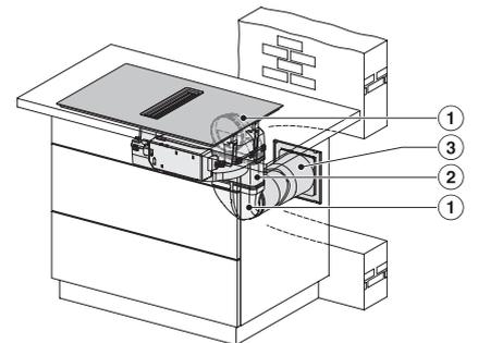
KMDA7676FL, KMDA7876FL – Installation variant 10 Exhaust air - drawing
