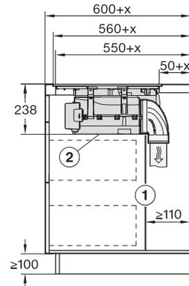
KMDA7676FL, KMDA7876FL – Side view flush+X – Installation drawing
