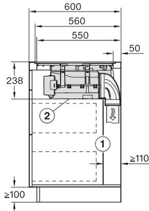
KMDA7676FL, KMDA7876FL – Side view flush – Installation drawing
