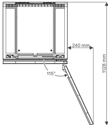
KWT6312UGS, KWT6322UG, KWT6322UG-1, KWT6322UG edt/cs (installation drawings)
