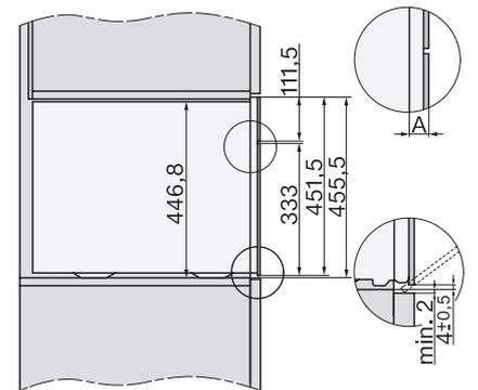
DGC7x6x X with and without handle side view, installation drawings
