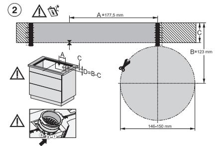
KMDA7272FL/FR, KMDA7473FL/FR – surface installation, drilling template, Installation drawing
