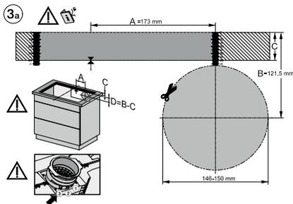
KMDA7272FL/FR, KMDA7473FL/FR – surface installation, 21 cm, drilling template, Installation drawing
