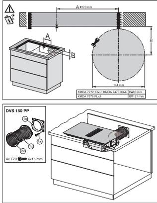
Installation plan DVS150PP – Installation drawing
