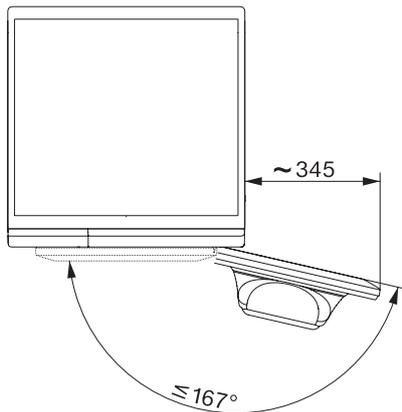
WT1 8/5 kg, drawing, slanted facia or straight facia, mesures in mm
