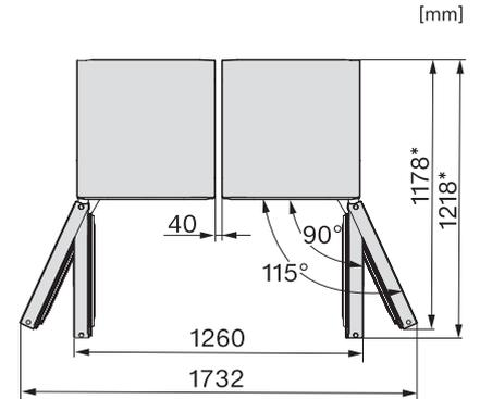
KS4383DD, KS4383ED, FNS4382E, FNS4382D, top view, Side-by-Side (footnote\*) (installation drawings)
