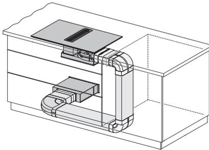
KMDA 7774, KMDA 7633 built-in version (Installation drawing)
