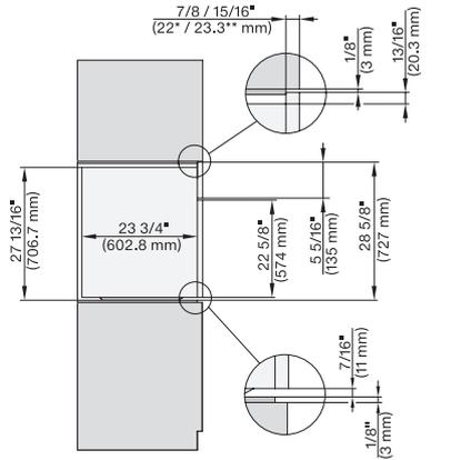
side view 30 inch Flush inset, installation drawing, NA
