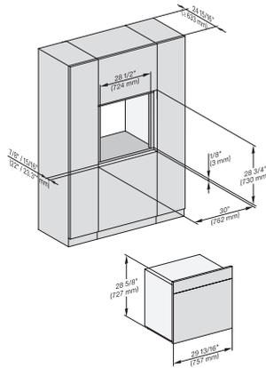
installation 30 inch Flush inset, installation drawing, NA
