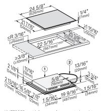
$\label{eq:KM7720FR} \mbox{KM7720FR} - \mbox{with frame, surface mounted overlying installation (*footnote)} - \mbox{drawing}$
