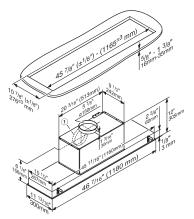
DA 2628, stainless steel – Integrated cooker hood (Installation drawing) – USA
