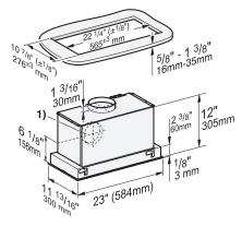
DA 2360 (Installation drawing) – USA 1) Vent connection alternatively to rear
