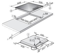
KM 3010 G (Installation drawing) 1. Front, 2. Casing depth, 3. Mains connection box with mains connection cable L = 2000 mmm, 4. Gas connection R 1/2" – ISO 7-1 (DIN EN 10226)
