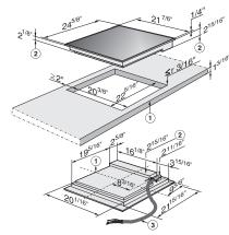
KM 5621 (Installation drawing) 1. Front, 2. Building-in depth, 3. Flexible metal hose, L = 1200 mm KM 5621 (Installation drawing) 1. Front, 2. Building-in depth, 3. Flexible metal hose, L = 47 1/4"
