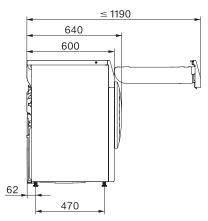
T1 installation drawing, slanted facia or straight facia, measures in mm
