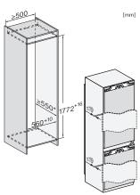
KFN7795D, KFN7795C, built-in (footnote\*) (installation drawings)
