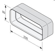
DFK-V, connecting plate, flat-type ducting, installation drawing
