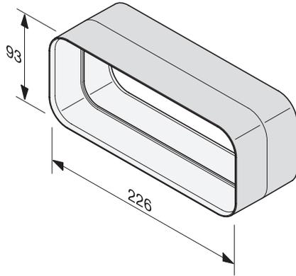
DFK-V, connecting plate, flat-type ducting, installation drawing
