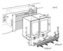
KWT6312UGS, KWT6322UG, KWT6322UG-1, KSK6300, Side by Side (installation drawing)
