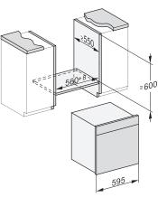
built-in DGC XXL build-under, installation drawing Worktop overhang  $\leq$  29 mm
