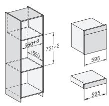
ESW7x10, EVS7010, DGC7x6xHCPro, DGC7x6xHCXPro installation drawings
