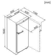
FN12621S-1, FN26062, FN26065 (installation drawings) (\*footnote)
