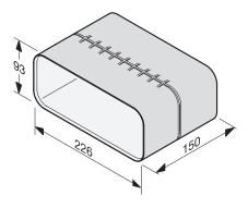
DFK-L Length adjustment 150 mm, Installation drawings
