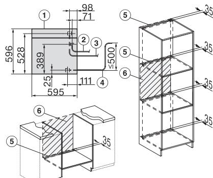
DGC7x6x connections and ventilation 60cm, installation drawing
