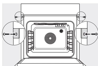
screw joint DGC XXL, installation drawing
