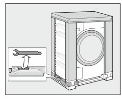
Take out the open spanner for removing the transit bars from the bottom left of the transport packaging.
