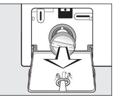
Remove the drain filter completely.
