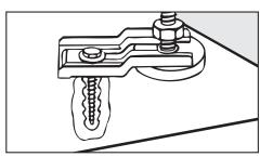
Fittings supplied are for installation on a concrete floor. For other types of flooring please purchase suitable fitting materials separately.
