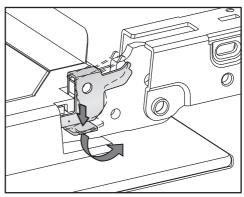
Release the locking clamps on the hinges by turning them upwards as far as they will go until they are at an angle.
