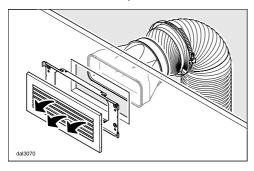
Conversion kit DUU 151 with a stainless steel grille is recommended if the grille is to be fitted in an area which is visible.
