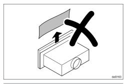
To avoid scratching the deflector plate, do not remove the protective film between the deflector plate and the casing until the hood has been placed in the housing unit.
