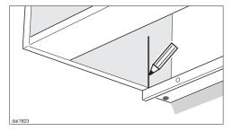
Draw a vertical line up both inside walls of the housing from the front of the spacer strip.
