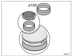
■ Attach the exhaust ducting, e.g. flexible hose, to the exhaust connection using a hose clip (available as an optional accessory).
