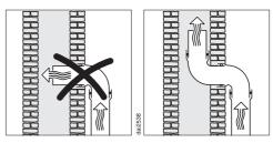
If the exhaust air is to be ducted into a flue, the ducting must be directed in the flow direction of the flue.
