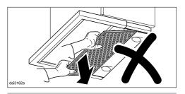
When removing the grease filter do not tilt it downwards at an angle. This can damage the retaining pins.
