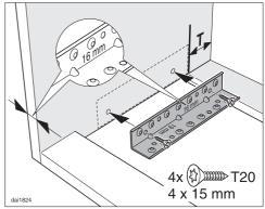
■ The brackets are designed for 16 and 19 mm thick unit sides. Orientate the bracket so that the vertical depth matches the thickness of the unit side.
