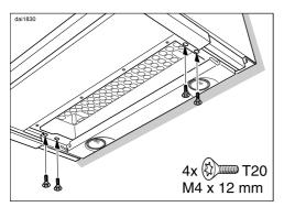
Secure the cooker hood to the brackets from below using two screws on each side.
