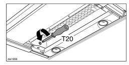
Note for dismantling the cooker hood: Undoing the screws on the left and right inside the housing releases the spring mounts allowing the appliance to be removed from the unit.
