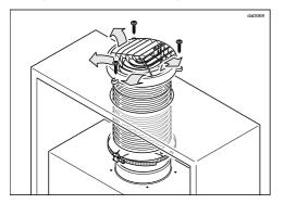
Conversion kit DUU 150 with a plastic grille is suitable for fitting in a nonvisible area at the top of the wall unit.
