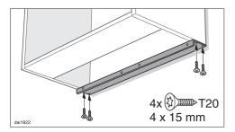
■ Secure the spacer strip underneath the housing unit sides, flush with the wall.
