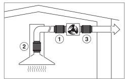
To minimise noise from the motor in the kitchen, the silencer should be positioned in front of the external motor ① if possible, or if the ducting is long, then in the ducting above the cooker hood itself ②. In the case of an external motor that is placed inside the house (ABLG 202), fitting a silencer behind the external motor ③ reduces the noise of the motor outside the house.
