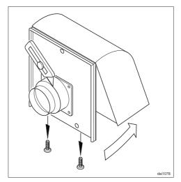
Unscrew the 2 fixing screws on the underside of the external motor and take the motor unit off of its fixing bracket.
