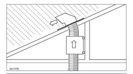
If the motor is installed vertically with the exhaust ducting venting over a roof, a roof vent kit DDF 125/150 or similar measures must be used to prevent the elements such as rainwater or snow penetrating the exhaust opening.
