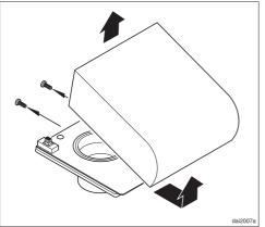
■ Unscrew the two fixing screws and remove the motor unit from the base plate.
