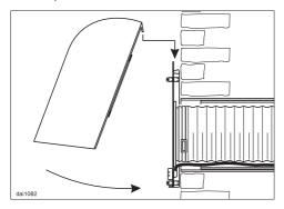
■ Refit the motor unit and secure with the 2 screws on the underside of the external motor.
