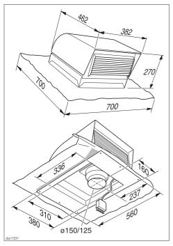
The DDG 102 is designed for installation on angled tiled, pantiled, slate or shingle roofs. The slope of the roof must be at least 22° to prevent the ingress of the elements, such as rain or snow.
