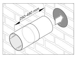
Push the telescopic wall pipe into the hole so that it is sitting flush.
