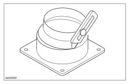
■ If a diameter of 150 mm is required, the front ring of the collar must be cut at the join with a sharp knife.
