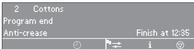
The program end is shown in the display and the buzzer sounds.
