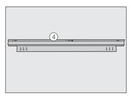
A bracket ④ (available from Miele) is required to secure the filler panel. The filler panel can be fitted above or below the appliance as required.
