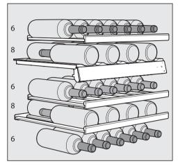
A total of 34 bottles (0.75 I Bordeaux bottles) can be stored in the appliance, with 14 in the upper section and 20 in the lower section.
