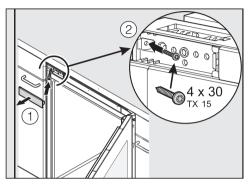
Remove the cover ① and first screw the appliance to the adjacent furniture unit at the top left ②.
