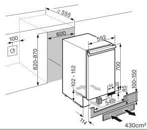
Before installation, ensure the building-in niche is the correct size. The specified ventilation cross-sections must be adhered to and the cut-out in the plinth facing for the ventilation grille supplied must be aligned centrally with the appliance in order to ensure the correct functioning of the appliance.
