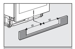
The cut-out in the plinth facing must be aligned centrally with the appliance.
