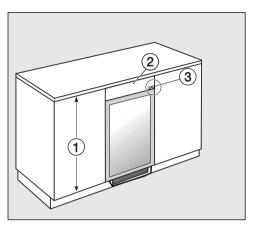
If adjacent furniture doors ① are taller than the wine conditioning unit door, the wine conditioning unit can be aligned to the unit doors using a filler panel ②.
