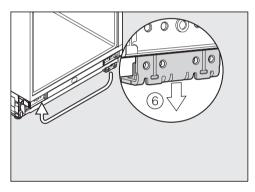
Remove the retaining bracket at the bottom right <sup>(6)</sup> of the appliance and fit it to the bottom left.
