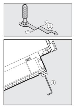
You can unscrew the adjusting feet using the spanner ③ supplied or an Allen key ④.
