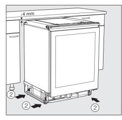
Unscrew the adjusting feet clockwise to 4 mm less than the height of the niche.
