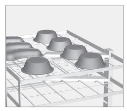
Containers e.g. beakers and kidney dishes should be placed in the mobile unit with the open side facing downwards, ensuring that all surfaces can be accessed easily and that cleaning solution can flow freely off them. They must also be secure so that they cannot be flipped over by the force of water during processing.
