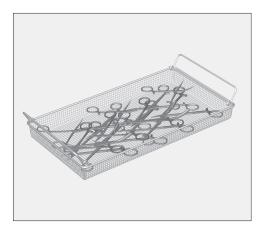
■ Hinged instruments must be opened up before being placed in the mesh travs to minimise the risk of surfaces not being accessed during processing.
