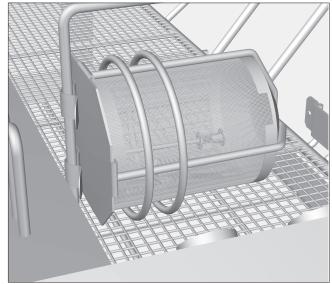
Place very small items (which could be washed through the mesh trays or through the gap between the mesh tray and the lid) in insert E 473/1 (available as an optional accessory).
