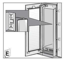
Now attach the covers onto the retaining clips on both sides.
