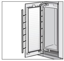
Fit the two plastic cover strips to the sides of the appliance door, clicking them into the space between the appliance door and the furniture front, starting at the bottom and working up to the top.
