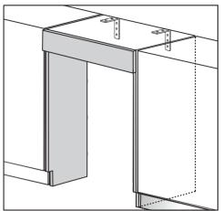
screw the building-in niche to the wall behind using a number of suitable angled fixing brackets. Use suitable wall plugs/fixing screws depending on the type of wall.
