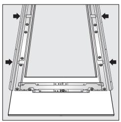
Insert the angle trim as far as it will go into the spaces in the frame, as shown.
