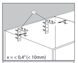
Danger of tipping. The building-in niche must be securely fixed to the wall behind using a number of screws to avoid the appliance tipping when it is fixed into the niche later.
