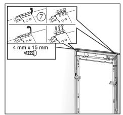
Pull out the lugs for the side fixing plates ⑦.
