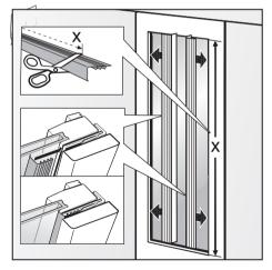
Trim the long pieces of door trim for the right and left sides to the length required X. Fix the door trim into the gap between the furniture front and the glass panel.
