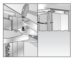
Insert the pin into the hinge from above, as shown.
