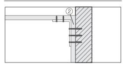
Use two anti-tipping mechanisms for each appliance or four for each side-by-side pair of appliances.
