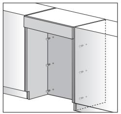
screw the back panel directly onto the wall behind in a number of places. Use suitable wall plugs/fixing screws depending on the type of wall. For a building-in niche **without** a back panel
