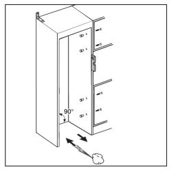
The building-in niche must be carefully aligned using a spirit level before installing the appliance. The corners must be at right angles, as otherwise the furniture door will not align correctly with the 4 corners of the building-in niche.
