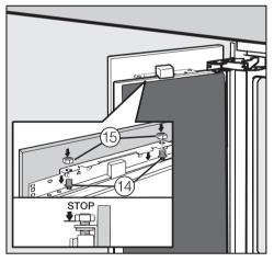
Open the appliance door and hang the furniture front on its frame onto the threaded bolts, as shown (4)
