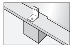
Unscrew the bracket that is holding the appliance to the delivery pallet.
