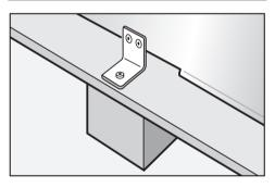
Unscrew the bracket that is holding the appliance to the delivery pallet.
