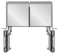
If the appliances are to be installed next to each other without a partition wall between them, they will need to be joined together using the side-by-side installation kit.
