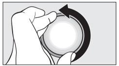
■ Turn the lamp cover anti-clockwise to remove it.
