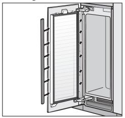
■ Fit the two cover strips to the sides of the appliance door, clicking them into the space between the appliance door and the furniture front, starting at the bottom and working up to the top.
