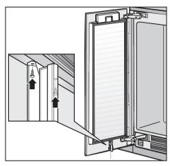
Screw the air separator to the middle of the appliance door using two screws.
