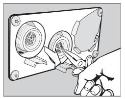
Use pointed pliers to grip the bar and pull out the filter; then clean the filter. Reassemble the appliance in reverse order.
