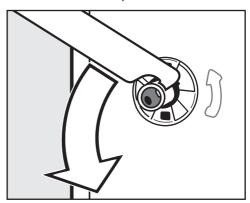
■ Using the wrench supplied, turn the left-hand shipping strut 90°.
