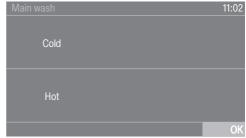
■ Touch the cold sensor control if the washing machine is only connected to a cold water supply, or touch hot if the washing machine is connected to cold and hot water.
