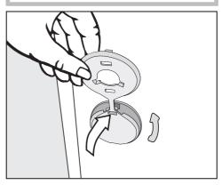
■ Install the covers onto the holes.
