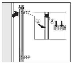
Secure the shipping struts to the back of the washing machine.
