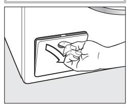
Open the access flap to the drain system.
