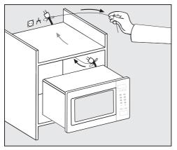
Slide the microwave oven into the housing unit. Feed the cable with the plug through the back of the unit.
