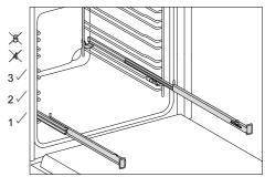
FlexiClip runners can only be fitted on levels 1, 2 and 3.
