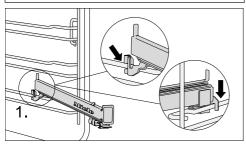
Hook the FlexiClip runner onto the front of the top rail of a side runner (1.).
