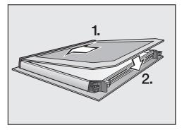
■ Push the inner pane with the matt printed side facing downwards into the plastic strip and place it between the retainers.
