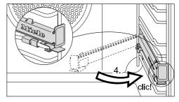
■ Then swing the FlexiClip runner back to the side of the oven compartment and secure it to the top rail with an audible click (4.).
