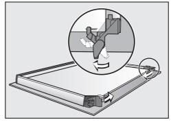
■ Flip both the glass pane retainers inwards in such a way that they fit over the lower of the two middle panes.
