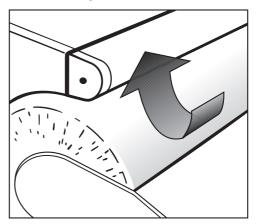
If you now lift the finger guard, the roller stops rotating and the heater plate rises up.
