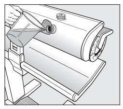
Before switching on, fill the water reservoir with tap water (approx.
