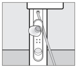
The screw-on funnel can be stored on the cable holder when not in use.
