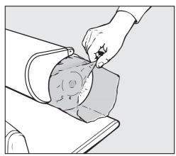
The protective dust cover can now be pulled out and off.
