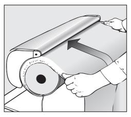
Press the foot pedal and "iron" the cloth into position.
