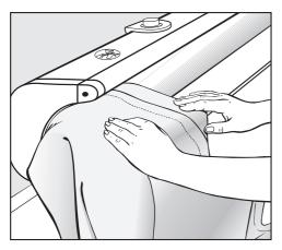
First do up poppers and buttons. Feed this end through the left hand side of the ironer first. Buttons should face into the roller.
