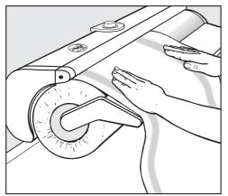
Then carefully turn the roller by hand until the laundry makes contact with the heater plate (keep your fingers away from the heater plate).
