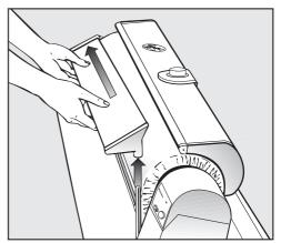
First lift it out of the right hand holder, and then pull it out to the left of the roller.
