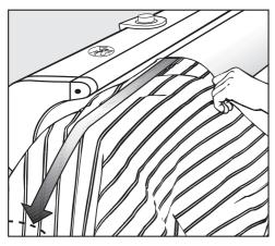
Pull the shirt over the roller as far as the yoke seam - or to the collar seam on shirts without a yoke - and smooth it out.
