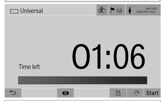
After selecting a programme, the time left for the chosen reprocessing programme is displayed. If the Display time left parameter is not activated in the web interface, the display switches to the already elapsed Duration of the reprocessing programme after programme start.
