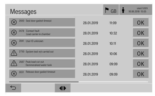
After a warning or fault symbol has been pressed in the main menu, the list containing all active messages is shown on the display. If the list contains more than 6 entries, a scroll bar will appear above the footer.
