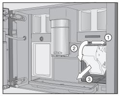
Pull the brew unit to the side ① first and then pull out to the front ②. Tilt the brew unit forwards ③. Clean the brew unit by hand under warm running water without using washing-up liquid or any other cleaning agent.
