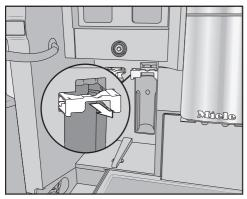
Pull the descaling cartridge holder forwards.
