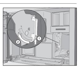
Press the button under the handle of the brew unit ① and, whilst doing so, turn the handle to the front ②.
