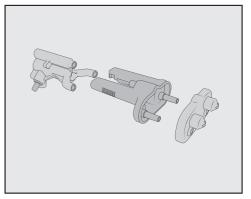
Dismantle the dispensing unit into three pieces: disconnect the Yshaped piece, the dispensing spouts and the holder from one another.
