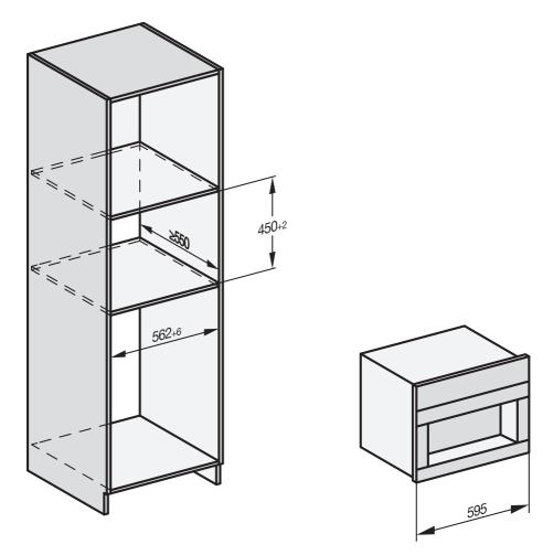
Combination with other Miele built-in appliances is possible. If the coffee machine is to be built in above another appliance, there must be a full-width, closed shelf between them. If the appliance is to be combined with a Gourmet warming drawer/built-in vacuum sealing drawer, no intermediate shelf is required in between.
