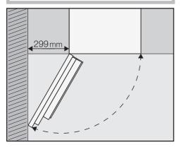
**Useful tip:** If the distance between an adjacent wall and the coffee machine is at least 299 mm, the appliance door can be opened wider, thus making the machine easier to use. This allows the left bean container to be removed more easily, for example.
