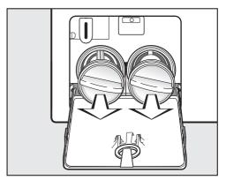
■ Remove the filters completely.
