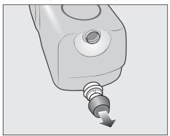
Remove the cover cap from the cartridge.
