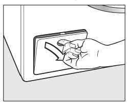
■ Open the drain pump access panel.
