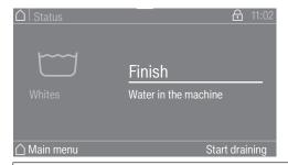
The suds are not drained so they can be used again in a subsequent program. Once the program has ended, the program end screen is displayed. It is possible to switch to the main menu while the suds are in the drum or to drain the suds by pressing the Start draining control. If permanent automatic water drainage is required, Automatic drainage can be activated at supervisor level.
