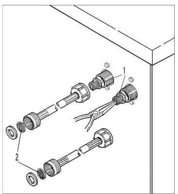
■ The filters in the water intake valves (1) and the inlet hoses (2) must be checked for soiling from time to time and cleaned as necessary.
