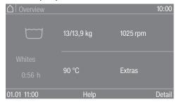
The program runtime will appear in the display either straight away or once the delay start period has elapsed. The program sequence is also shown in the display.
