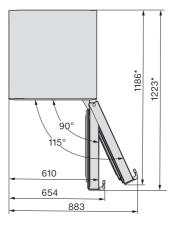
$^{\star}$  Dimensions without wall spacers fitted. Fitting the wall spacers supplied increases the appliance depth by 15 mm.
