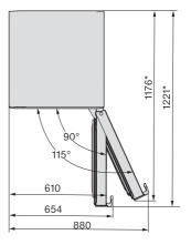
\* Dimensions without wall spacers fitted. Appliance depth is increased by 15 mm with the wall spacers supplied fitted.
