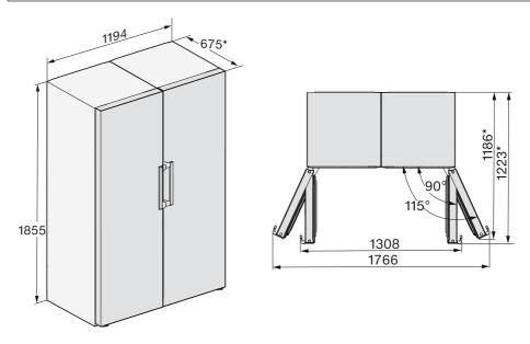
\* Dimensions without wall spacers fitted. Fitting the wall spacers supplied increases the appliance depth by 15 mm.
