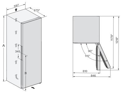
$\star$  Dimensions without wall spacers fitted. Appliance depth is increased by 15 mm with the wall spacers supplied fitted.
