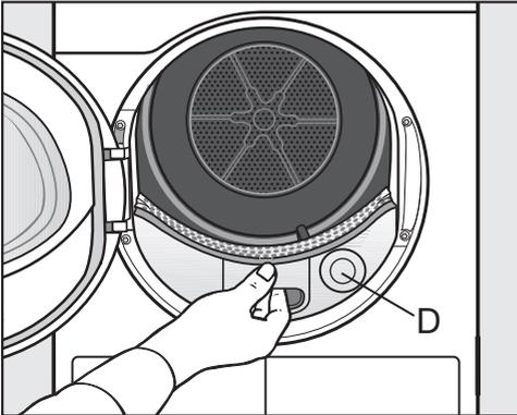
The round cover (D) has no function and cannot be removed.
