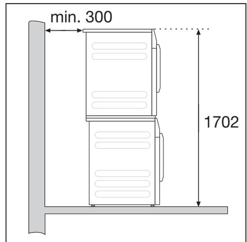
A stacking kit\* is required. This must be fitted by a Miele authorised service technician.
