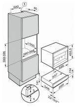
ESW 6114, ESW 6214 (Installation drawing) \* appliances with glass front \*\* Appliances with metal front
